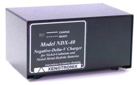
negative-delta-V sensing with 12.5-bit resolution, digital filtering, currentless voltage sensing, and a nominal –0.5% (with respect to top level) negative-delta-V detection level. To prevent the false detection of negative-delta-V, the sensing circuit is inhibited at the beginning of the charge cycle. The back-up timer is matched to four charging rates: 2C (45 min), 1C (1.5 hr), 0.5C (3 hr), and 0.25C (6 hr).
